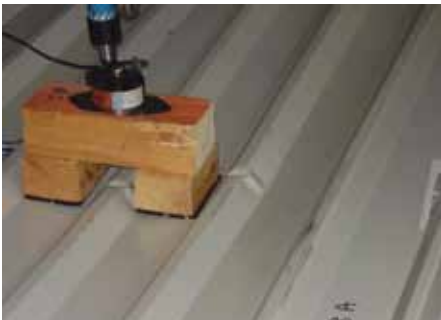
Figure 8. Resistance to concentrated forces test in progress
