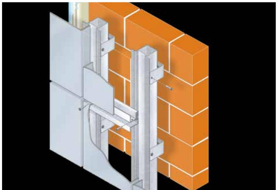
Figure 13. Pre-finished steel rainscreen cladding system
