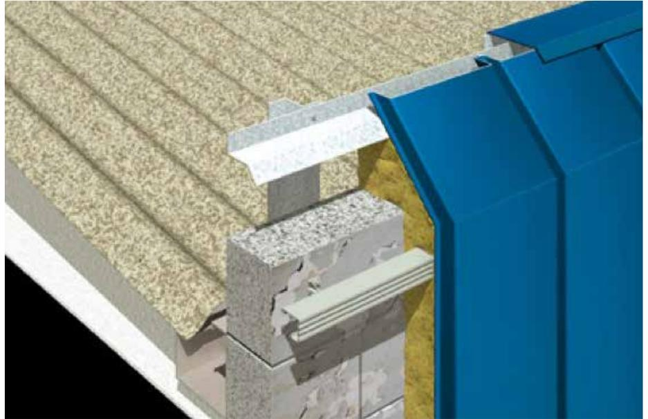
Figure 8. Pre-finished steel flat profile and trapezoidal profile over cladding wall systems
