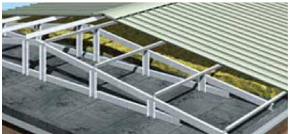
Figure 20. Typical construction detail of roof cladding and the supporting structure
