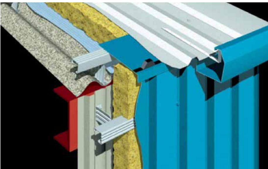
Figure 7. Through fix pre-finished steel profile insulated over cladding system
