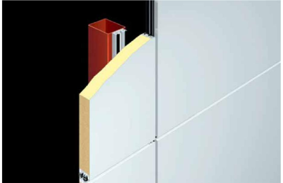
Figure 12. Pre-finished steel flat panel façade system
