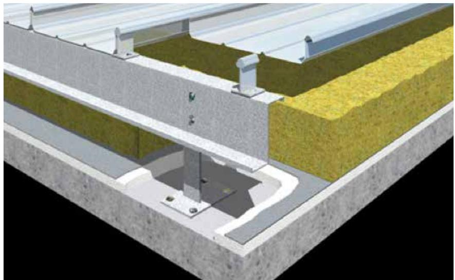
Figure 11. Pre-finished steel standing seam pitched over cladding system
