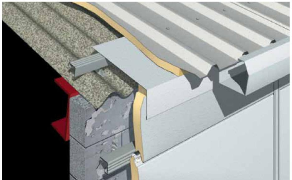
Figure 9. Pre-finished steel composite panels for roofs and walls
