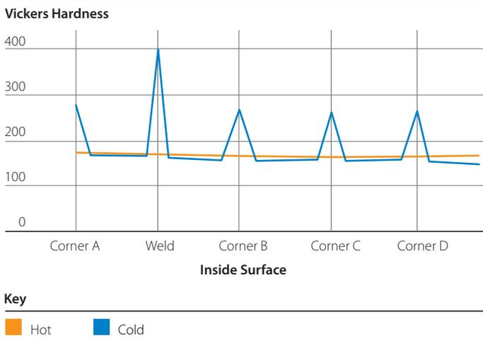
Typical plot of hardness values on inside surface of square structural hollow sections.
