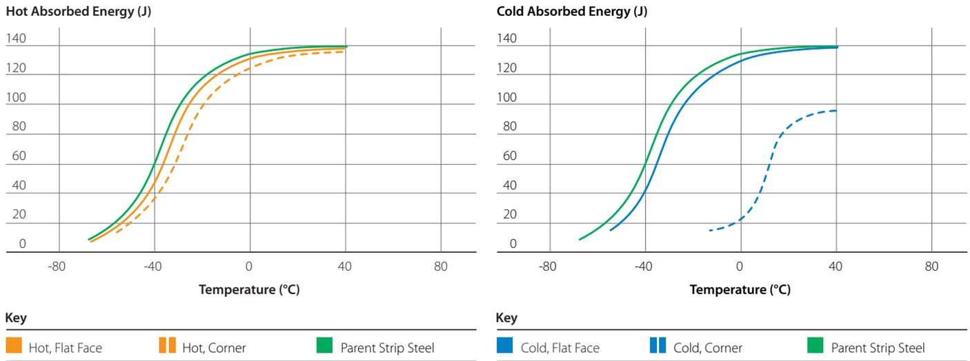
Typical Charpy toughness: temperature graph for specimens taken from structural hollow sections.
