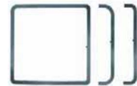
Photograph comparing corner radii, from left to right, in hot-finished, cold-formed stress-relieved and cold-formed structural hollow sections.
