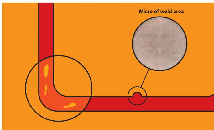
**Celsius®355** has uniform grain structure with low hardness.
