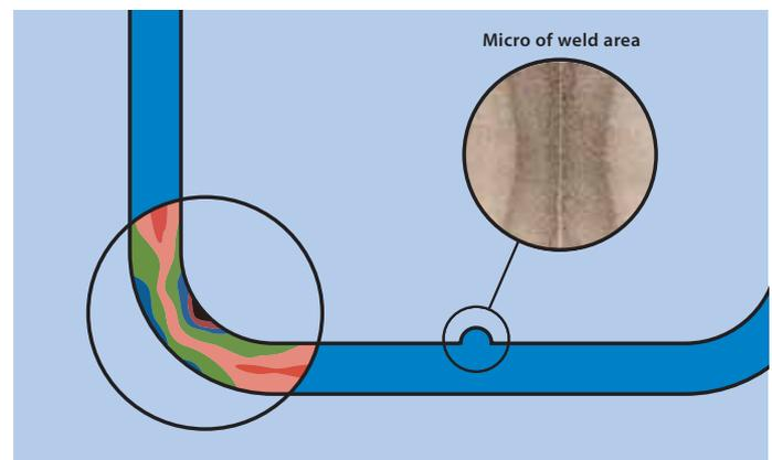
Cold-formed structural hollow sections have varying grain structure with hardness peaks.
