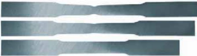
Photograph of stages of the tensile test indicating ductility achieved by test specimen taken from **Celsius®355**.
