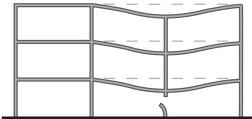
Frames can be designed to exhibit ductile behaviour, offering alternative load paths in the event of unexpected removal of columns.
