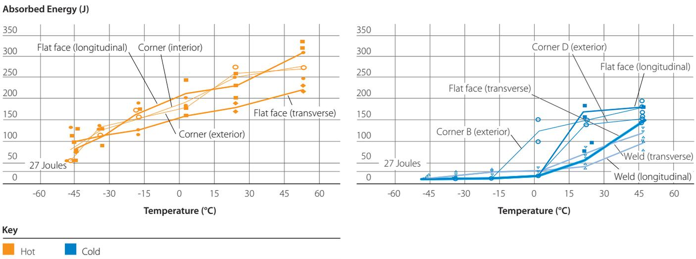
Charpy toughness versus temperature plots for specimens taken on flat faces, in longitudinal and transverse directions, at welds and in corners (see Footnote 2).
