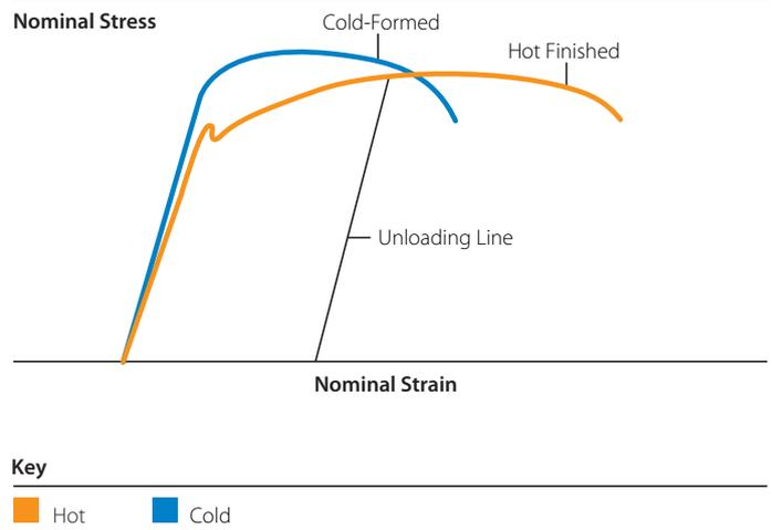
Schematic stress: strain plots for test specimens taken from corners of Celsius® 355 and cold-formed structural hollow sections indicating differences in ductility.
