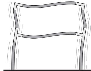
Moment frames can be designed to have ductile and energy-absorbing characteristics under extreme loading conditions.
