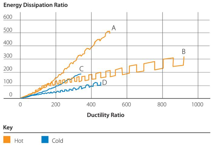
Energy dissipation versus ductility plots for X-joints under reverse loading. This indicates superior performance of the hot-finished sections (see Footnote 1).
