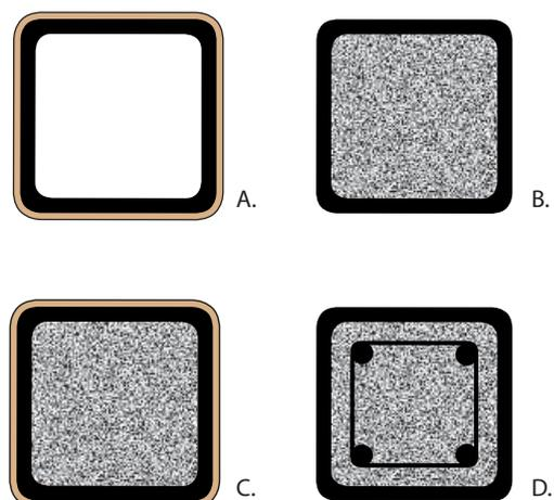
Fire resistance may be achieved by A. Intumescent external protection, B. Concrete filling of the inside, C. Filling together with an intumescent external protection or D. Concrete filling with reinforcement.
