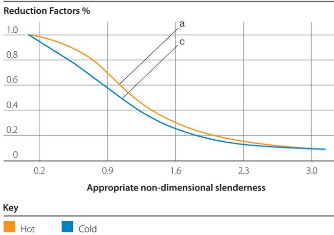
Buckling curves from EC3 Part 1.1 showing 'a' curve for hot-finished and 'c' curve for cold-formed structural hollow sections.
