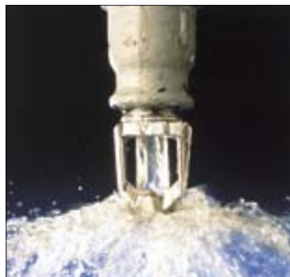
Figure 11 Sprinkler head exploding. Courtesy of Wormald Ltd.
