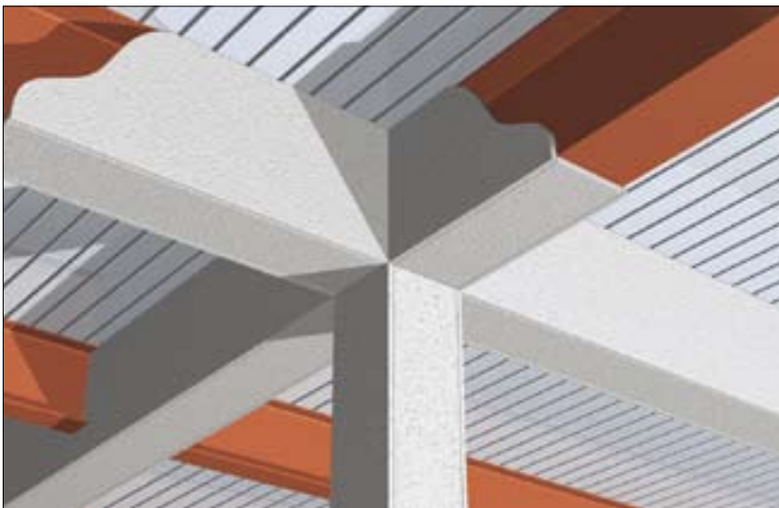
Figure 23 Fibre board applied to beams.
