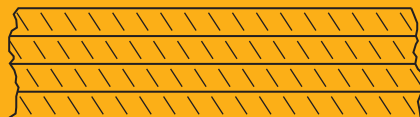
Figure 1 Example of rib pattern of grade 460A with four transverse rib series.
