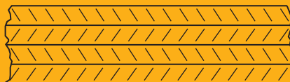
Figure 2 Example of rib pattern of grade 460B with four transverse rib series.
