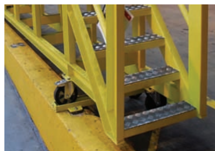
Wheel guide track support used on uneven ground
