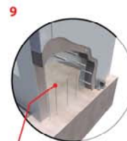
9 Rebar set into foundation (by others), centred between Bi-Steel connecting bars
