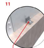
11 Angle weld to Bi-Steel panel to accept holding down bolt cast into foundation
