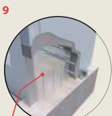
9 Rebar set into foundation (by others), centred between Bi-Steel connecting bars
